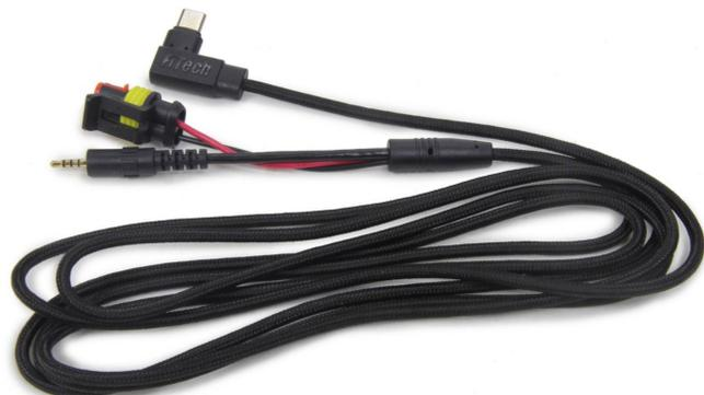
**Handheld Controller Cable:** Connects the ECU to the Handheld. The 2-wire connection on the harness supplies constant battery 12 Volts and ground to the Handheld. The stereo jack connector has the K-Line CAN communication line. The USB-C connection of the Handheld harness can be inserted into either the bottom of the Handheld or Handheld dongle.
