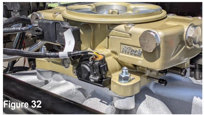
**TPS:** This connector connects onto the throttle position sensor mounted on the driver's side of the throttle body.
