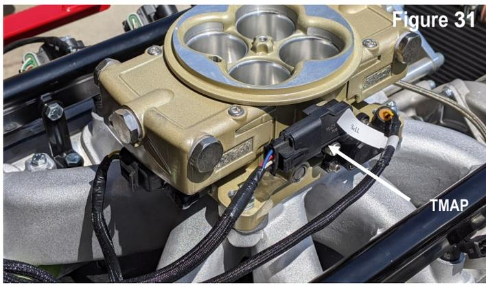
**TMAP:** Connects to the temperature/manifold absolute pressure (TMAP) sensor mounted on the side of throttle body. Sensor is pre-assembled onto throttle body from factory.
